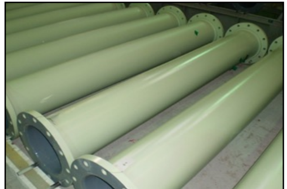
Finished pipes ready for service coating with ARC S2 .
